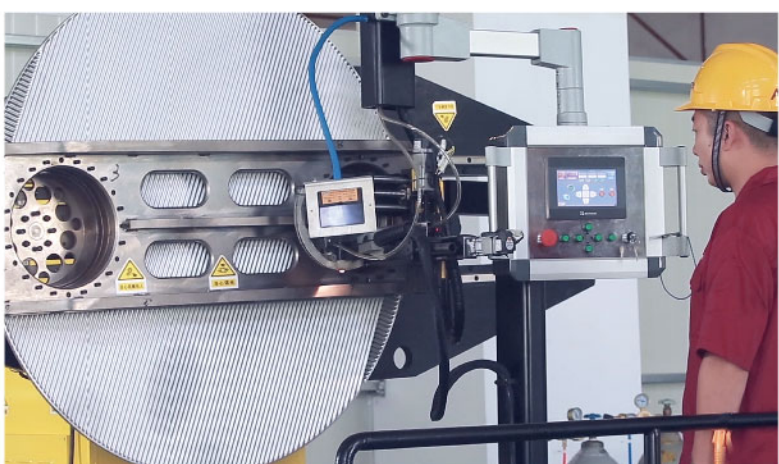
Automatic plate welding (AWPS)
