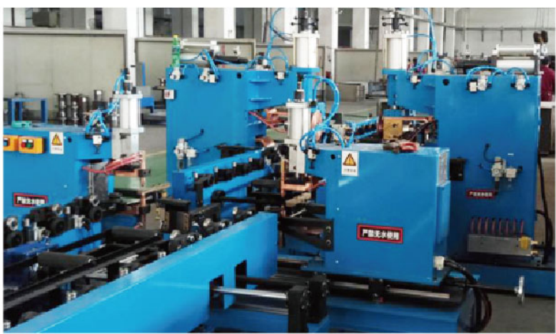
Automatic plate welding (AWK)
