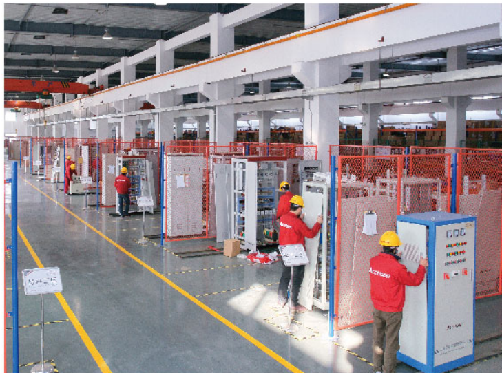
Electric control cabinet production line
